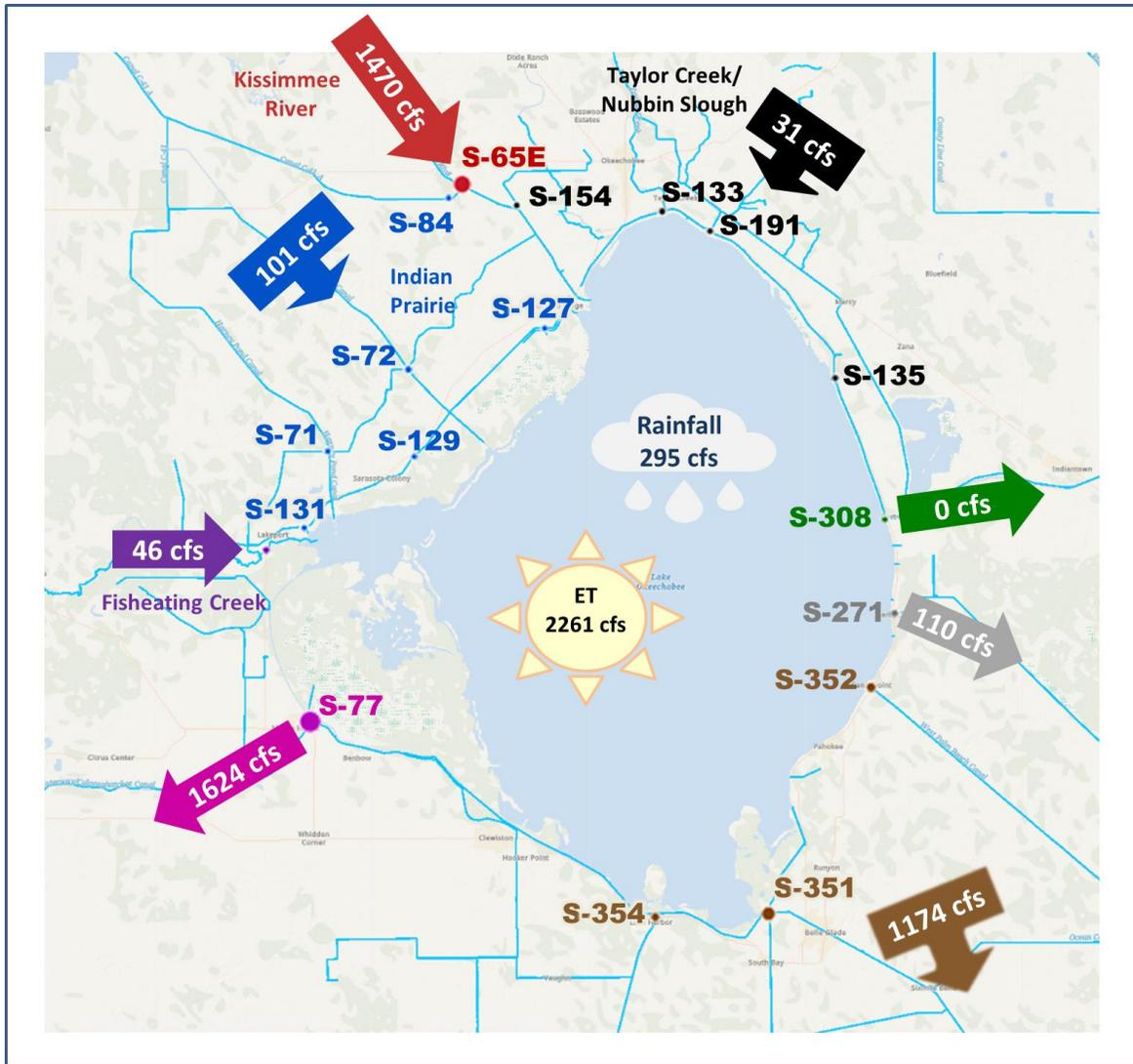
**Figure LO-5.** Inflows into Lake Okeechobee from Indian Prairie basins, Taylor Creek/Nubbin Slough, Kissimmee River and Fisheating Creek, and outflows to the west via S-77, to the east via S-308, to the south via S-351, S-352, S-354, and to southeast via S-271 (formerly Culvert 10A) for the week of January 09 - 15, 2023.
